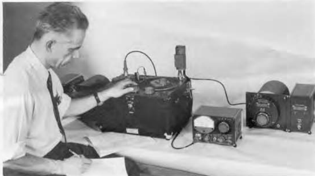
Type DNT-5 Heterodyne Detector in use with the Type 916-AL RF Bridge.
